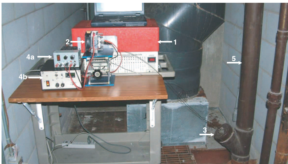
Figure 5. Illustration of toluene monitoring in a sewer pipe at the Department of Chemistry in the University of Waterloo: 1: SRI8610GC; 2: microtrap in control unit; 3: membrane module inside the sewer pipe; 4: power for the cooler (a) and the heater (b).
